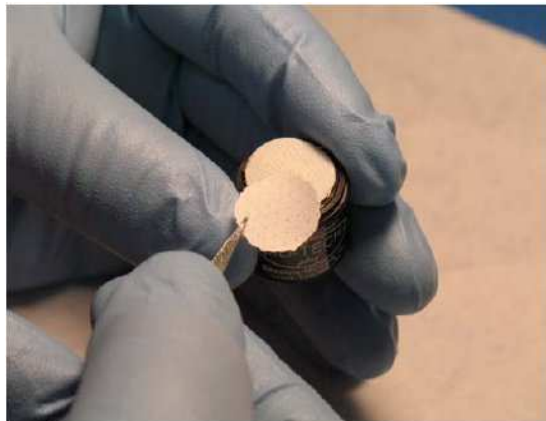
Figure 29 Installing Filter Media
