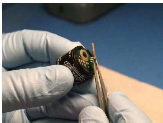
Figure 27 Cell Assembly installation
